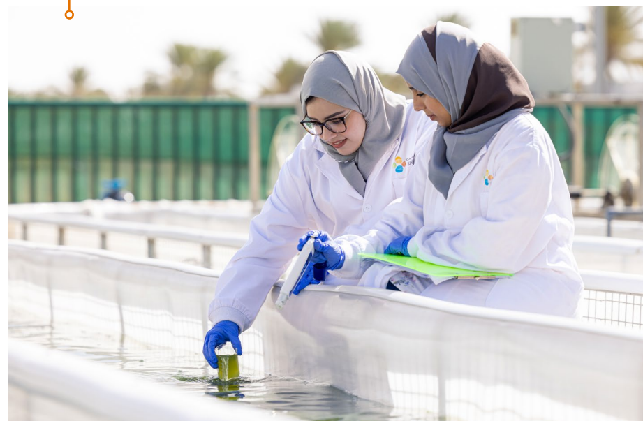
DABKSA staff measuring main abiotic parameters in production raceways (open systems) at pilot plant facilities
